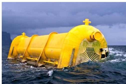
The Oyster 800 wave-energy device, in operation at the European Marine Energy Centre's (EMEC's) Billia Croo site https://undark.org/2024/04/29/scotland-ocean-power/
